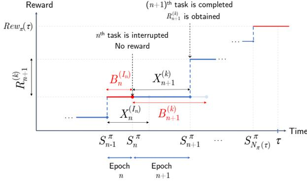
Fig. 1. Illustration of a sample path for the BwI process. The completion time  $X_n^{(I_n)}$  of the  $n$ -th task exceeds the interrupt time  $B_n^{(I_n)}$ , so the task is interrupted. In the  $(n + 1)$ -th epoch, arm  $k$  is chosen, and the task is completed before the interrupt time, yielding a reward of  $R_{n+1}^{(k)}$ .
